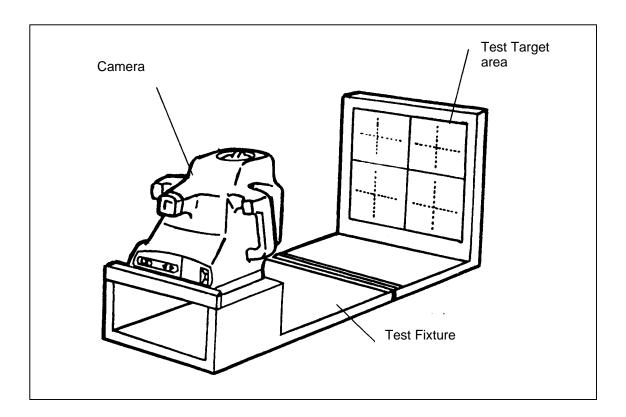
Figure 3-1 Camera Test Fixture
